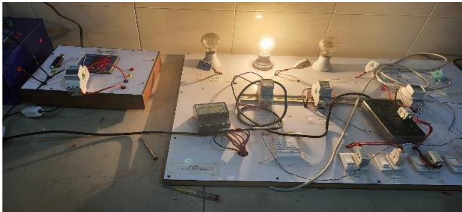
Fig 1: SME 104 Smart meter collecting data
